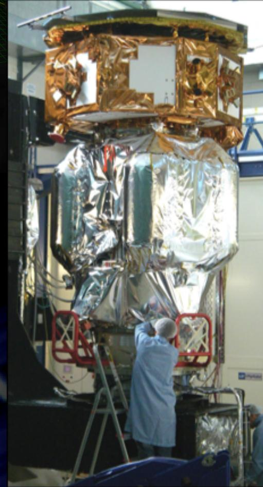
Transfer orbit thermal tests
